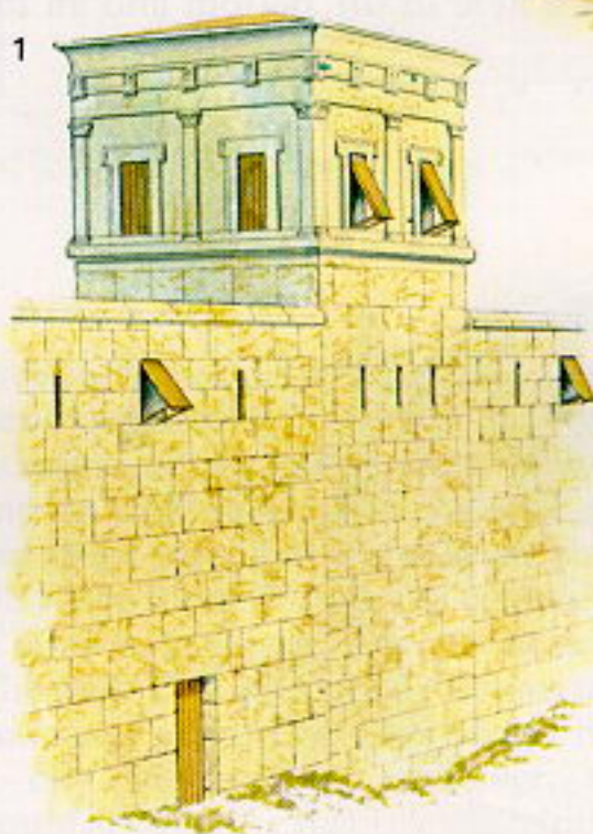
Above A reconstruction of part of the walls and a tower at Paestum (after Krischen). The tower had shuttered windows and loopholes for catapults, but no crenellations on the tower or walls.
