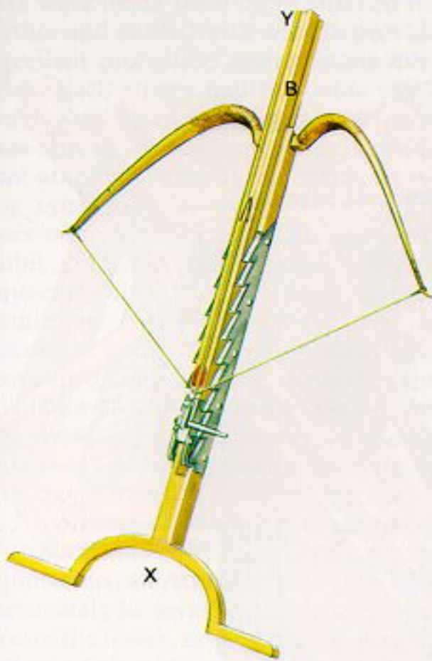
Above The earliest catapult—the belly bow ( gastrophetes ). The bow was drawn by placing X round the belly. Y on the ground and using the weight of the body to force back the slider B —hence its name. After E. W. Marsden.
