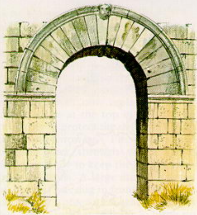
Above Etrusco-Roman arched gate, at Santa Maria di Falleri. Below Wall of polygonal masonry, Segni. When this masonry was used, gateways often had sloping sides and were either pointed at the top or had a long lintel across.
